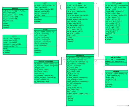
Figure 3. Class Diagram
