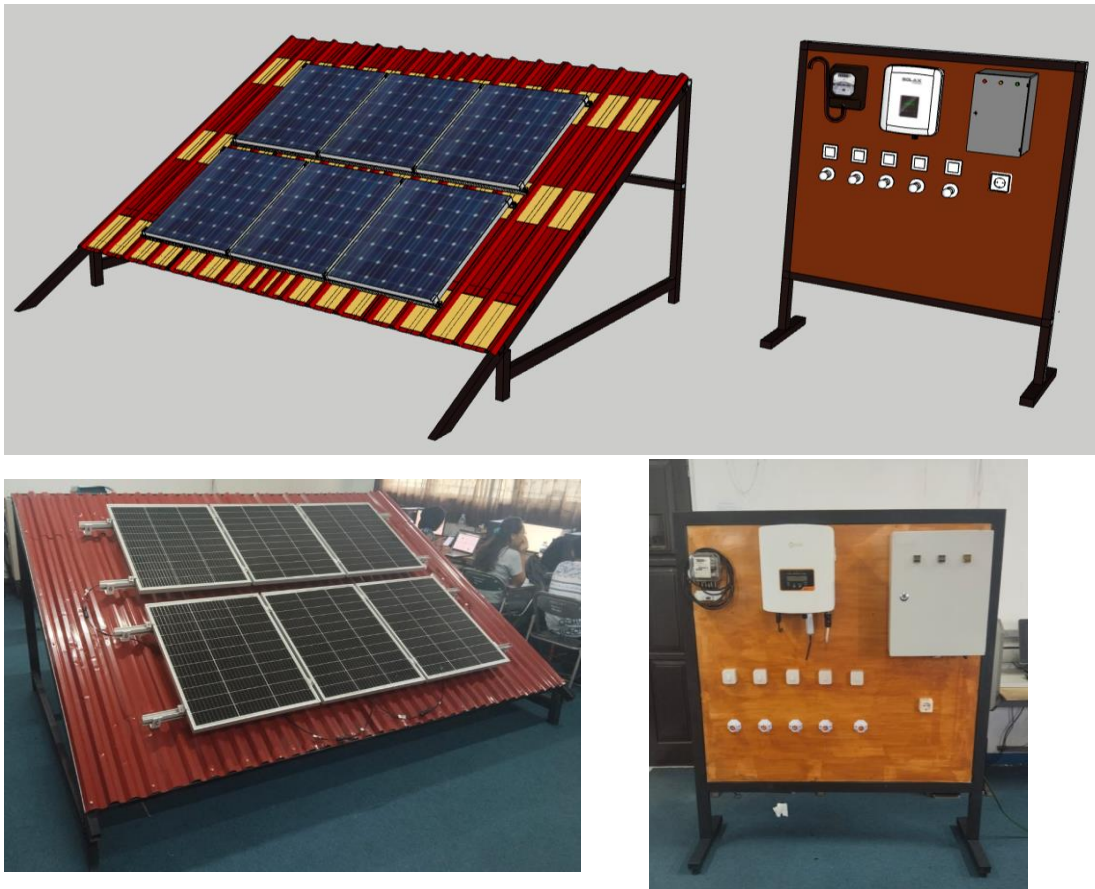
Figure 1. Design of rooftop PV system training equipment
