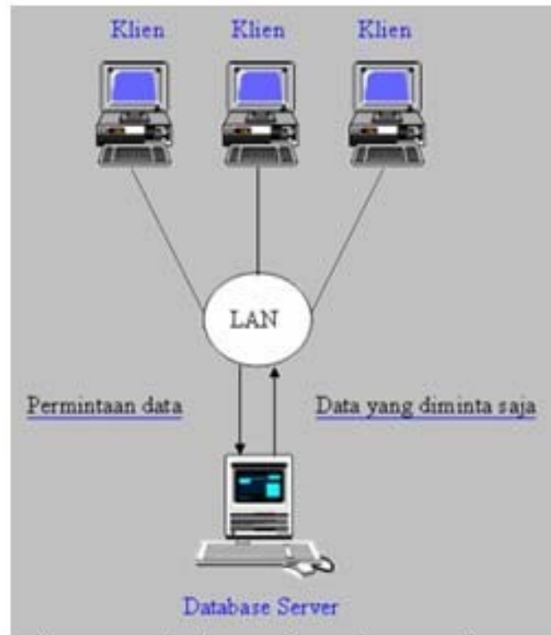
Gambar 3. Arsitektur Client-Server (Two-Tier)
